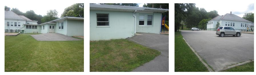
Stormwater is currently directed to an existing detention basin. Parking spots on the southwest side of the building can be replaced with porous asphalt to capture and infiltrate stormwater. A rain garden adjacent to the building can capture, treat, and infiltrate roof runoff. A preliminary soil assessment suggests that the soils have suitable drainage characteristics for green infrastructure.
