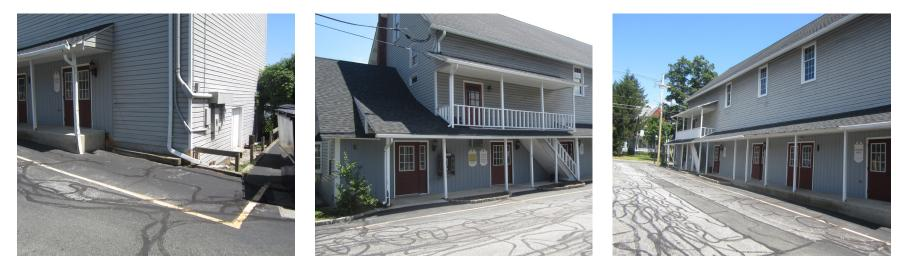
Stormwater currently drains toward the rear of the building. Three downspout planter boxes adjacent to the building can capture, treat, and infiltrate roof runoff. A preliminary soil assessment suggests that the soils have suitable drainage characteristics for green infrastructure.
