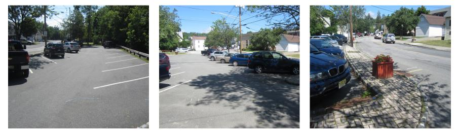
Stormwater is currently directed to an existing catch basin. Parking spots on the north side of the lot can be replaced with porous asphalt to capture and infiltrate stormwater. A preliminary soil assessment suggests that the soils have suitable drainage characteristics for green infrastructure.
