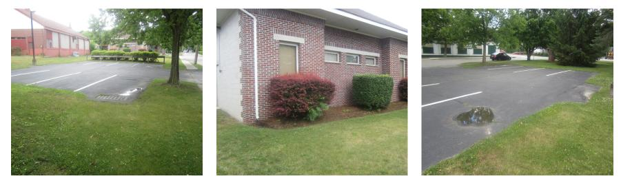
Stormwater is currently directed to an existing catch basin and the local sewer system. Parking spots in both the south and the north parking lot can be replaced with porous asphalt to capture and infiltrate stormwater. A rain garden adjacent to the building can capture, treat, and infiltrate roof runoff. A preliminary soil assessment suggests that the soils have suitable drainage characteristics for green infrastructure.
