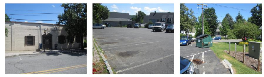
Stormwater is currently directed to an existing catch basin. Parking spots in the rear parking lot can be replaced with porous asphalt to capture and infiltrate stormwater. A preliminary soil assessment suggests that the soils have suitable drainage characteristics for green infrastructure.
