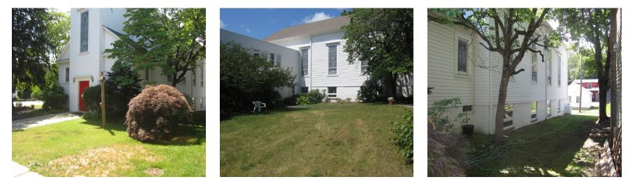
Stormwater is currently directed to the west side of the building where it is the cause of erosion issues. Rain gardens adjacent to the building can capture, treat, and infiltrate roof runoff. A preliminary soil assessment suggests that the soils have suitable drainage characteristics for green infrastructure.
